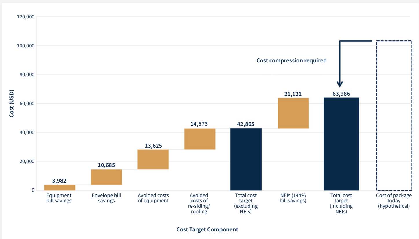
Exhibit 27. Illustrative Cost Target Breakdown for the “Equipment + IECC Envelope” Package for Single-Family Homes
