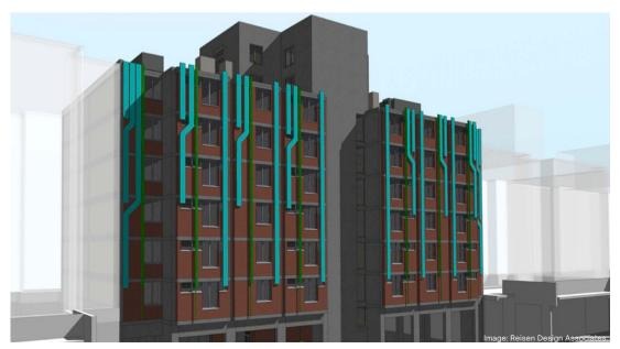
New refrigerant lines and supply ductwork along façade before panel installation.
